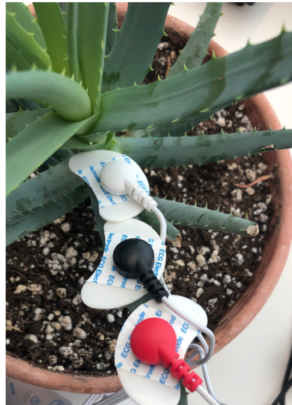
Surface-mounted electrodes on plant
